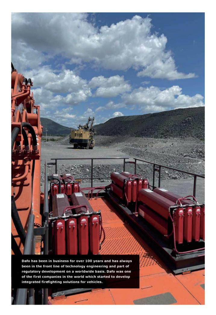
Mining, both surface and underground, is a complex operation that needs large offroad vehicles/ heavy duty mobile equipment (HDME) and processing equipment that operate at remote locations 24/7. In addition, these machines operate under challenging and demanding conditions in environments with many potential fire hazards as the HDMEs often carry a lot of ammable liquids in pressurized fuel lines close to hot engines and transmissions.
